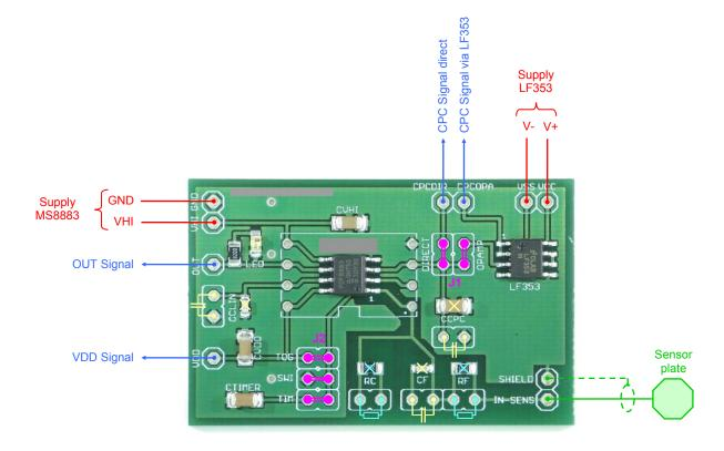
The pre-assembled SMD resistors and capacitors may be changed in order to experiment with the set-up. In addition, the SMD components may be removed and conventional components may be soldered on to the board in the positions that are marked in yellow and turquoise. The component labels are marked between the corresponding connections. The sensor compensation section covers the effects of changing the component values.
